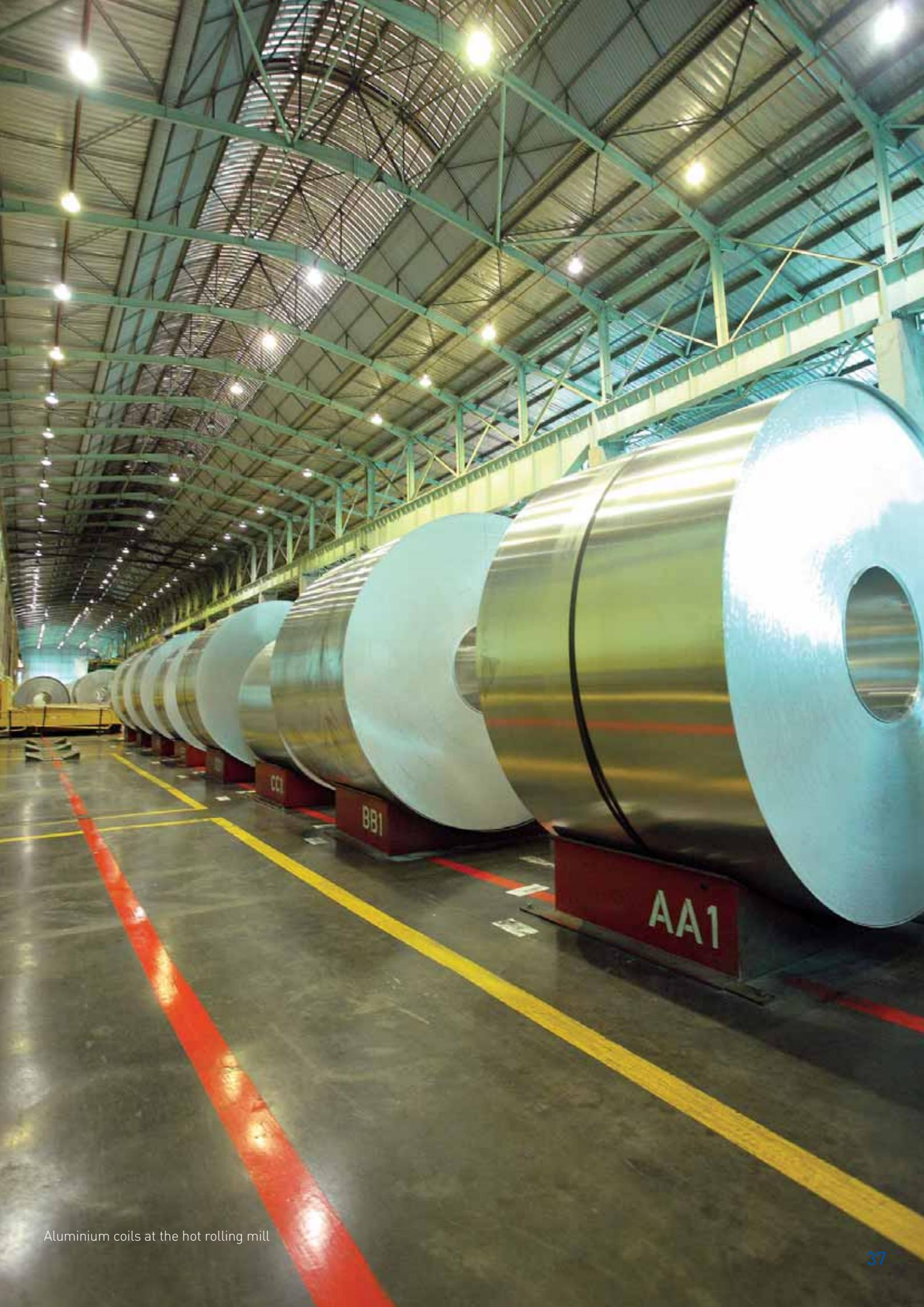
Aluminium coils at the hot rolling mill
