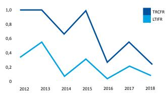
The Total Recordable Case Frequency Rate (TRCFR) and the Lost Time Injuries Frequency Rate (LTIFR) is the number of recordable injuries divided by the number of hours worked, multiplied by 200 000. Targets for 2018 were LTIFR 0.05 and TRCFR 0.5.
